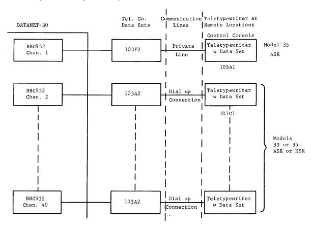
Figure 1. Interface Communications Hardware
