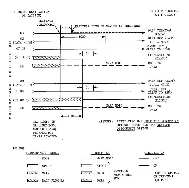
Figure 5. Data Set 103A Space Disconnect Sequence
