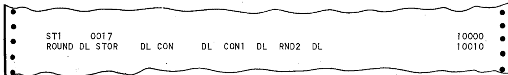
Figure VII-11. Special Symbol Table as Produced by a Punched Card System and Listed on the High-Speed Printer by a Magnetic Tape Assembly Program
